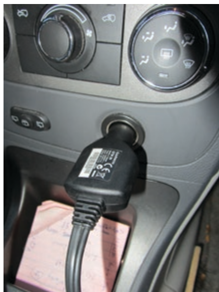
Splicing a 12V DC power outlet plug in place of the router's AC/DC adapter provides a fast, weather-proof, and always there power solution.
