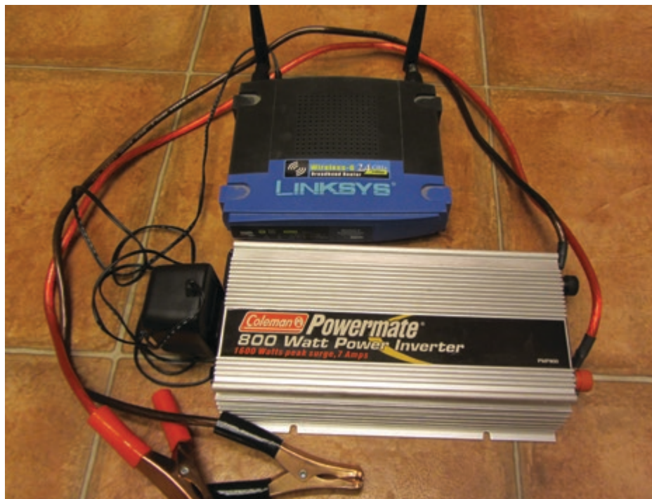
The heart of a WIFI range setup is shown, a router and inverter sans battery.
